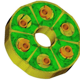
Flexible coupling disc | FEA
